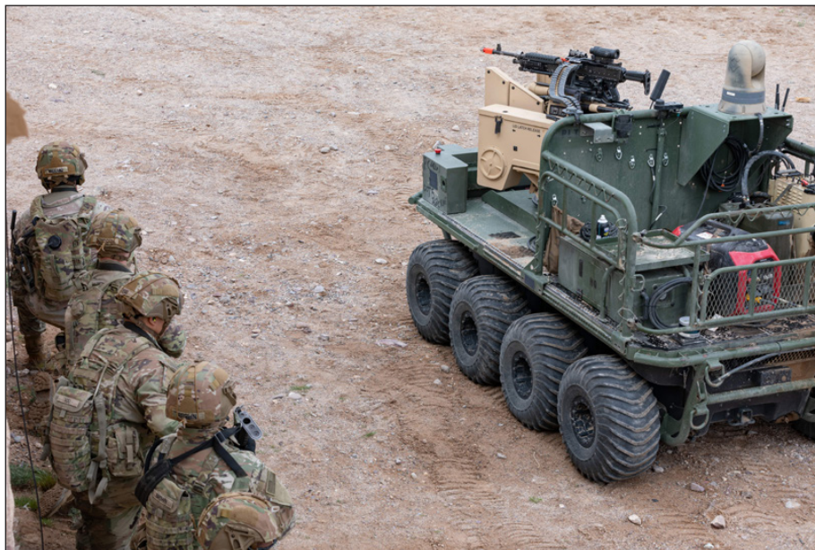
A U.S. Army unmanned, eight-wheeled, all-electric, all-terrain transport vehicle armed with the R600 autonomous weapon system provides support to dismounted Soldiers as part of a human integration experiment. (Photo by SPC Samarion Hicks)
